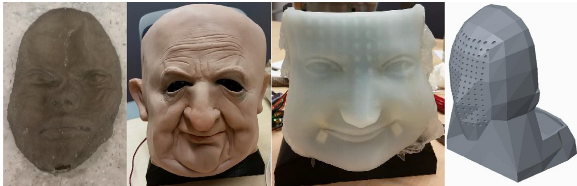
Fig. 17. From left to right: (1) mask 3D printed from TangoBlack+, (2) happy expression with off-the-shelf latex mask on generic skull, (3) happy expression with silicone mask on generic skull, (4) 3D printed generic skull.
