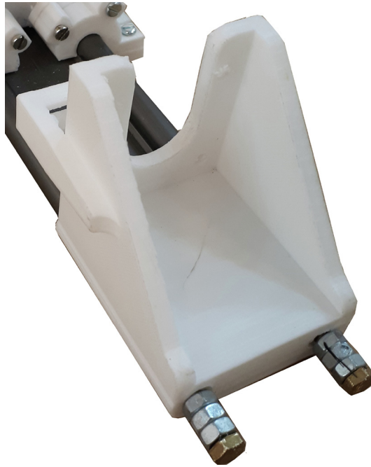
Fig. 3. The method for attaching the motor holder with the limit switch holder.
