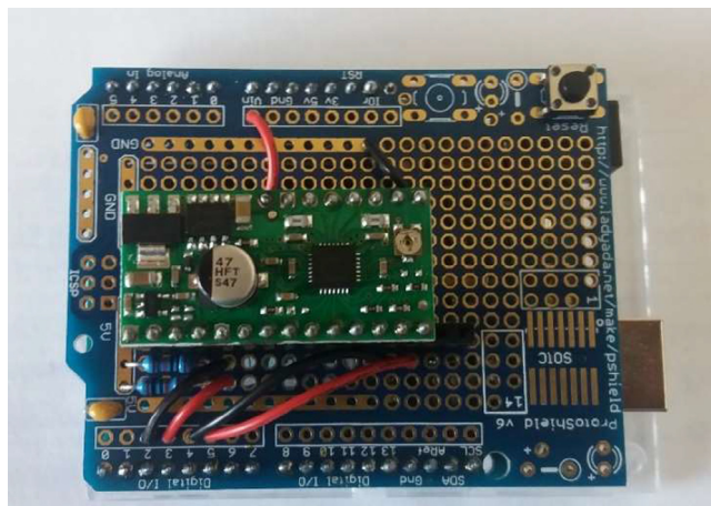
Fig. 4. The Arduino protoshield is connected to the Arduino UNO through male-to-male header pins, and the motor driver and resistors are soldered onto the protoshield.
