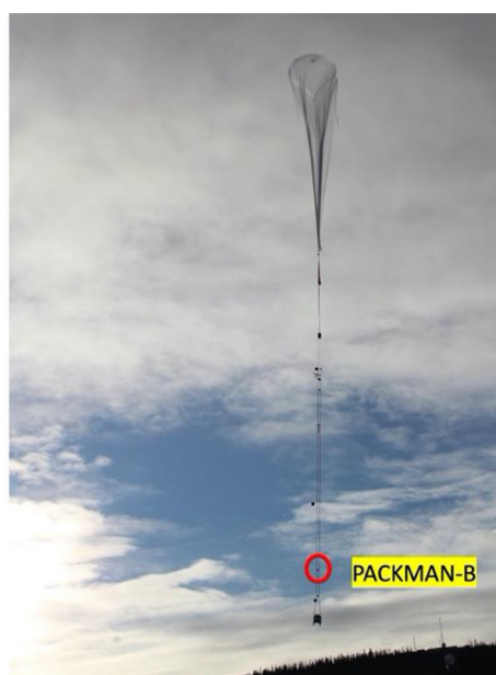
Fig. 11. PACKMAN-B payload attached to the tether of the stratospheric balloon during its launch from Esrange Space Centre, Kiruna.
