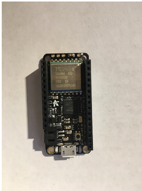
Fig. 35. Top view after soldering female headers on the Development Board.
