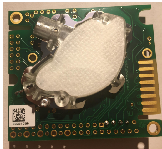
Fig. 12. Top view of the CO 2 Sensor after soldering 4-pin male headers.
