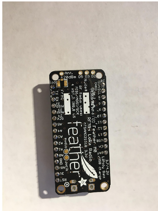
Fig. 36. Bottom view after soldering female headers on the Development Board.
