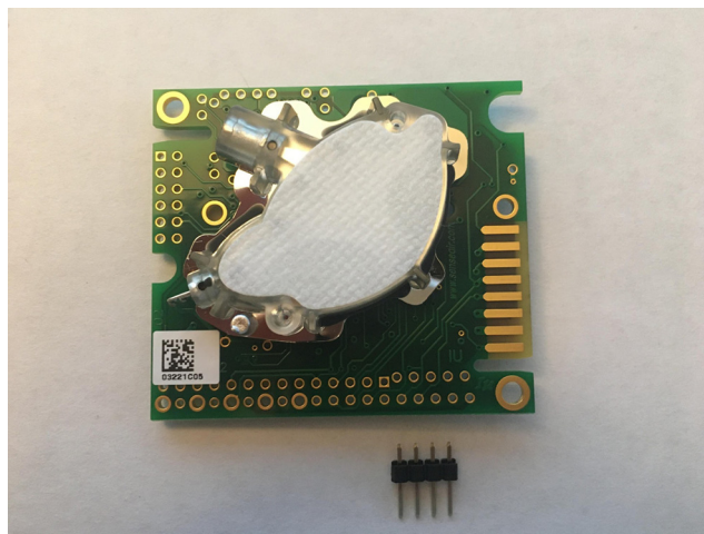
Fig. 10. The CO 2 Sensor and 4-pin male headers.
