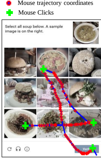
Figure 2: An application example of our proposed mouse bot detection algorithm in combination with a traditional image-based CAPTCHA. While the user completes the image CAPTCHA task (cognitive challenge), our algorithm analyzes the mouse trajectories performed during the task (neuromotor challenge).
