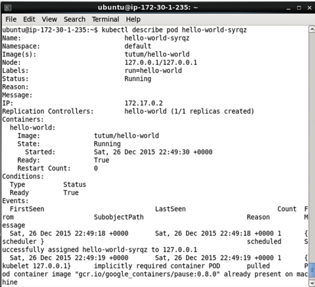
Figure 2-8. Describing a Pod
