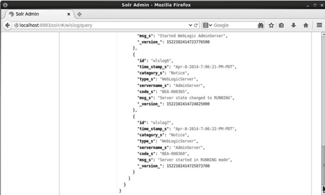
Figure 11-41. The _version_ field is added to each document stored in Solr index automatically by the Solr server
