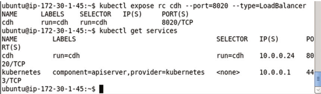
Figure 10-51. Creating a Service
