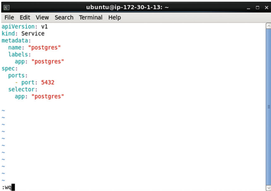
Figure 5-4. Service Definition File postgres-service.yaml
