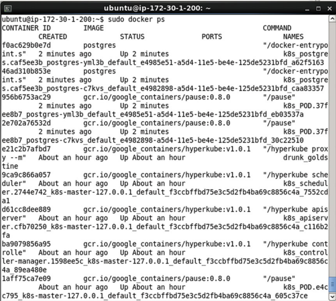
Figure 5-30. Listing the Docker Containers
