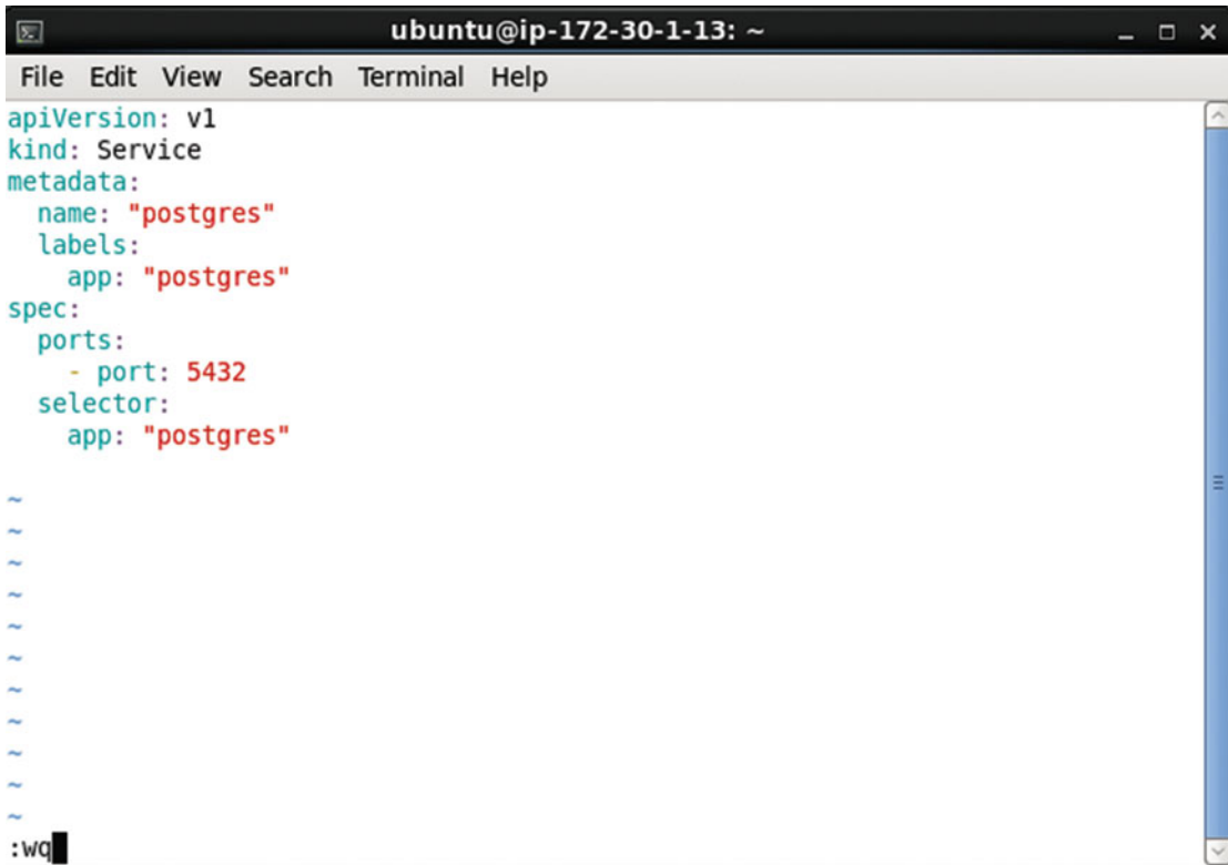
Figure 5-4. Service Definition File postgres-service.yaml
