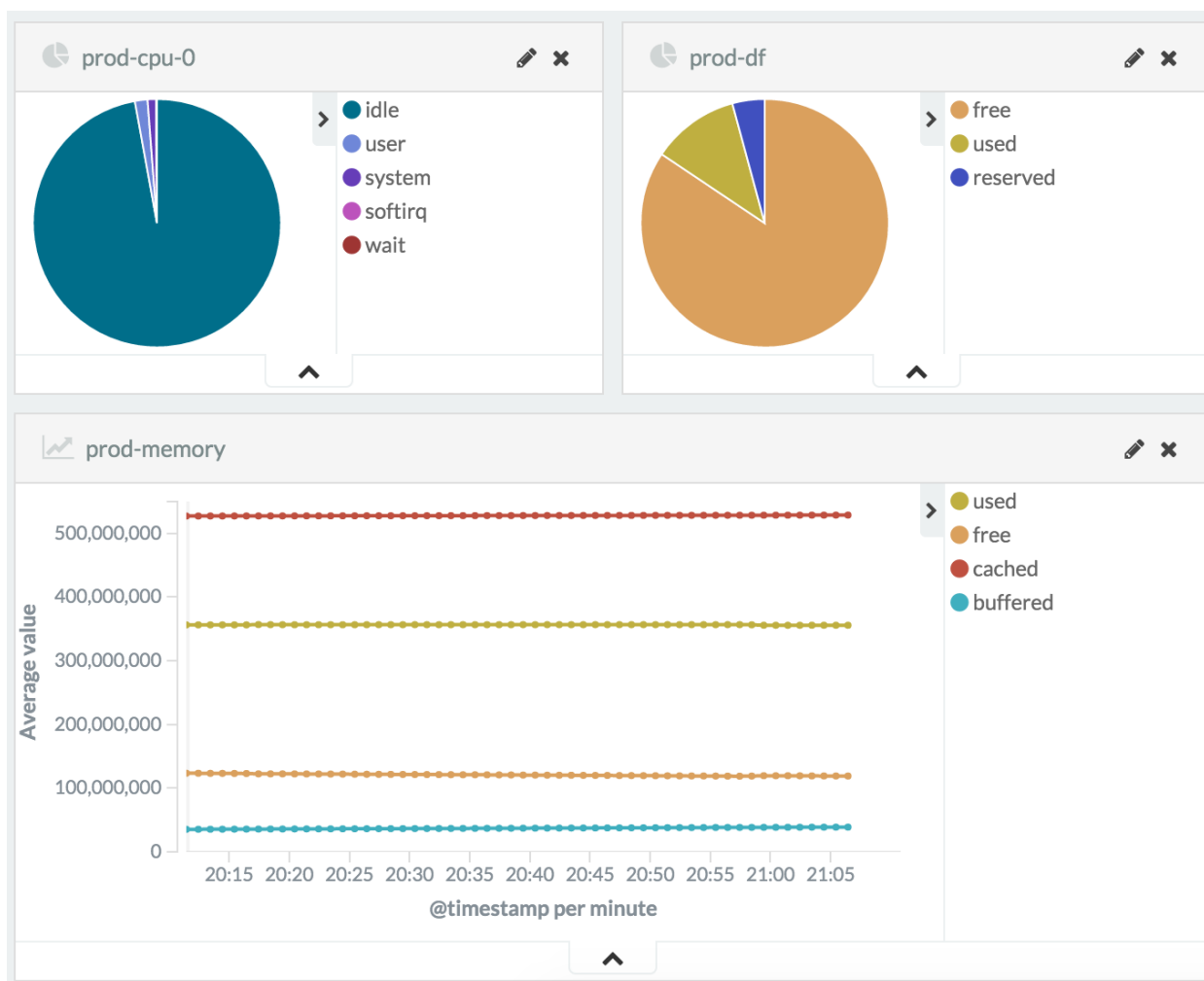
Figure 16-08: Kibana dashboard with CPU, hard disk, and memory usage over time
